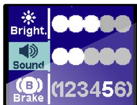
Display brightness, beeper volume and braking level can be adjusted in the Settings menu
