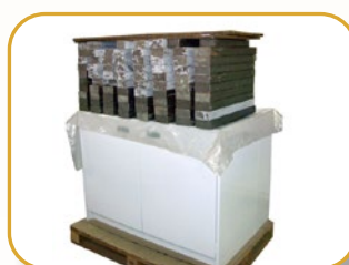
Actual photo during Cabinet Load Testing
